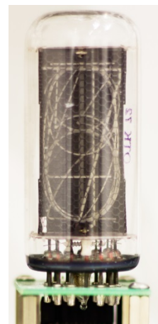
Figure 5: Nixie tube on prototype artwork (IN-18) © Rachel Ara 2014
